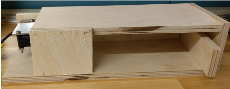
Figure 10: Laser interface prototype. The extra piece of plywood on the right side is used to alter the measurement during testing.
