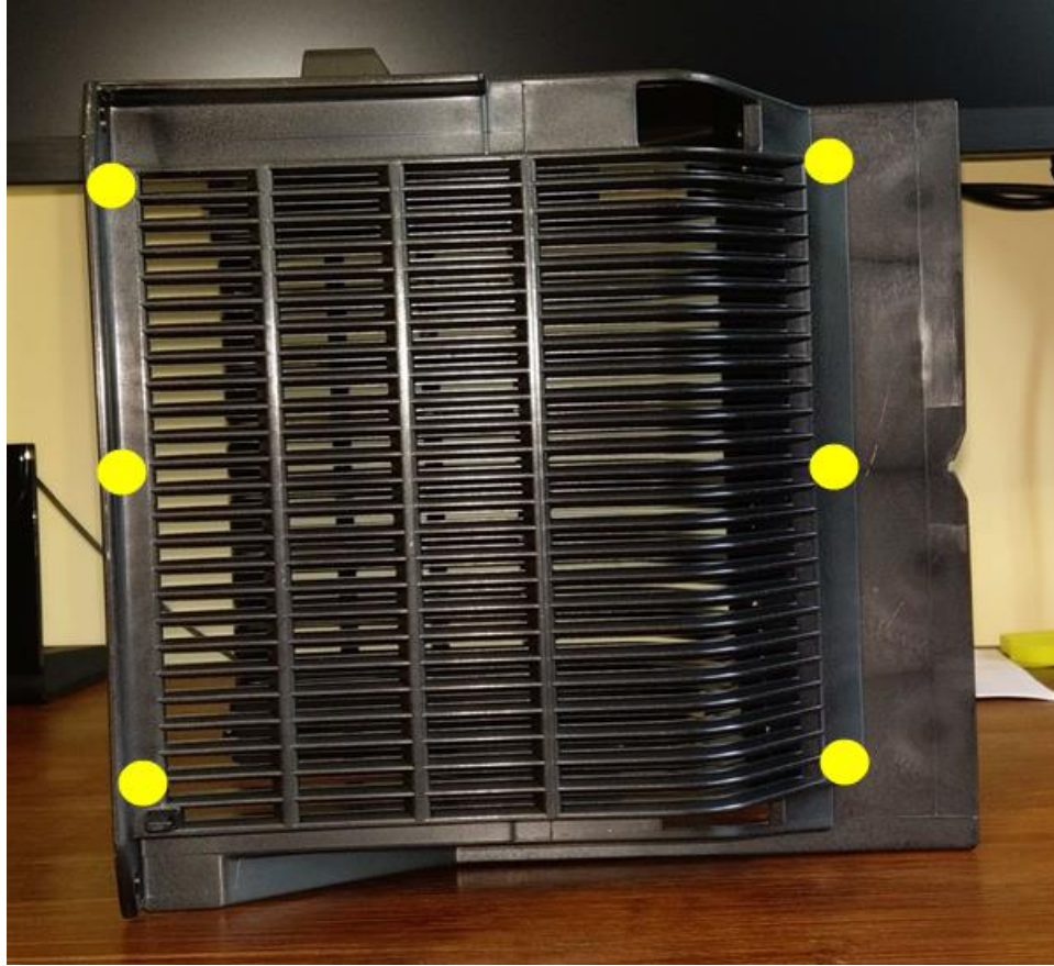
Figure 9: The key measurement locations to identify the lean condition marked by the yellow dots.
