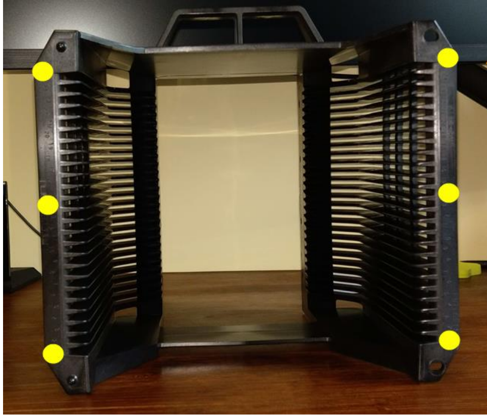
Figure 8: The key measurement locations to identify the twist condition as marked by the yellow dots.
