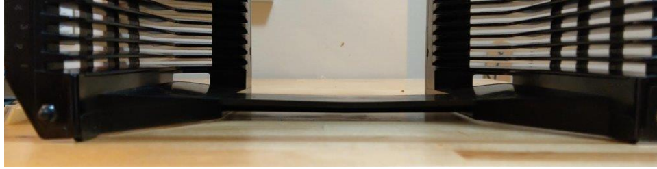
Figure 7: Bottom of the cassette viewed from the front showing the H-Bar bridging the gap between either side.
