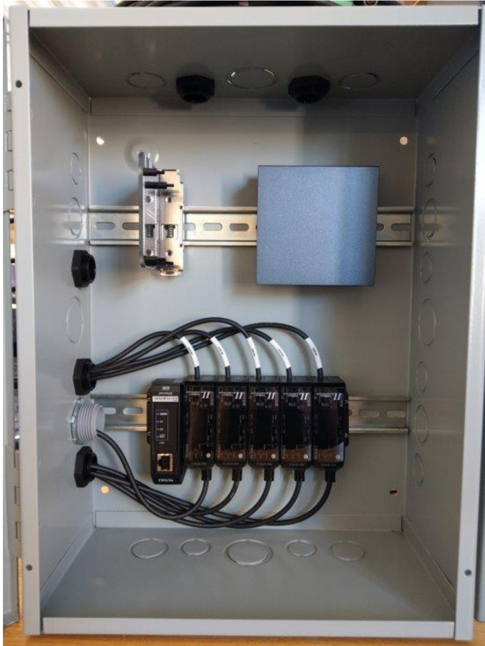
Figure 22: Front Hoffman Box Wiring. From top to bottom rail: microcontroller mount and networking switch, laser amplifier.
